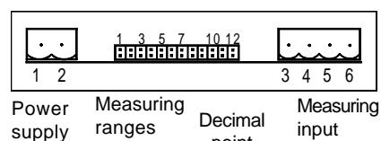
Power supply      Measuring ranges      Decimal point      Measuring input
